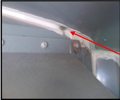
If a leak has occurred a visual check will show a clean area on the bin wall that is usually dusty. This is caused by an air stream coming through the bin divider and blowing product from a section of the wall around the leak area.
