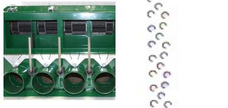
Metering Unit vanes positioned to mix 'N' FERTILISER with 'P' FERTILISER in Lines 1 & 3
