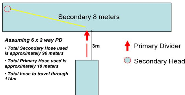
The diagram on the left shows a primary divider fitted at the centre rear of the cultivator. In this example, with a wide implement, the secondary hoses will be far in excess of the recommended five metres. In this case the primary dividers should be moved out further onto the implement, positioned as not to clash with folding, and as shown in the example below.
