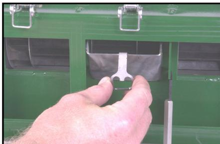
Spool Covers are easily installed by removing the front panel on the metering unit and placing the spool cover in front of the spool to be blanked off or restricted as shown. Push the cover firmly in until it clips into place.
