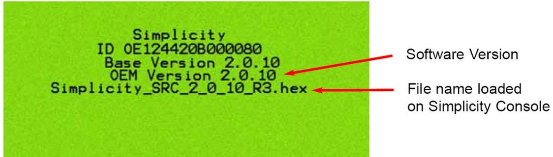
The above screen is displayed for 60 seconds each time the Seeder Console is switched on using the 'power' switch. It is not necessary to have this information displayed for the full 60 seconds if not required. When the screen is displayed simply push the 'enter' button to move into the working screen.
