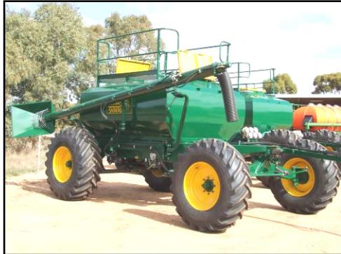
Load/Unload auger in the stowed position
