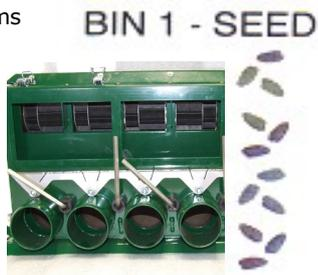
Metering Unit vanes positioned to direct 'P' FERTILISER into air streams 1 – 4, mixing with seed in air streams 2 & 4
