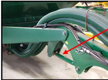
**N.B.** The threaded link on the Air Seeder Pull should be adjusted to keep the Seeder level when operating. Once the correct length has been attained it is important to tighten the two locking nuts at either end of the link to retain adjustment.
