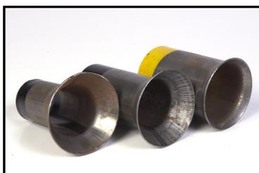
50 mm restrictors are supplied standard with the Air Seeder. Restrictors of different sizes are available from your Simplicity Australia Dealer. Experimenting with different size restrictors may be required to balance the air flow in some circumstances.
