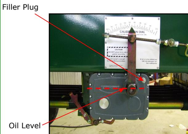
The 'Zero Max' drive is factory lubricated and mostly maintenance free. The oil level should be checked at the start of the sowing season. Remove the filler plug and check that the oil level is at the mid point of the upper most shaft as shown.
