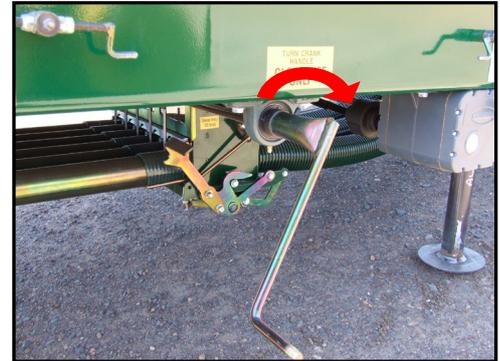
**Step 9.** Record the weight of the product metered and enter into the Simplicity E15 Actuator Drive Seed Rate Controller as per the Actuator Drive Seed Rate Controller Operators Manual. The 'Calibration Factor', which is the relationship between the calibration shaft turns and the weight of the product metered, is then automatically calculated.
