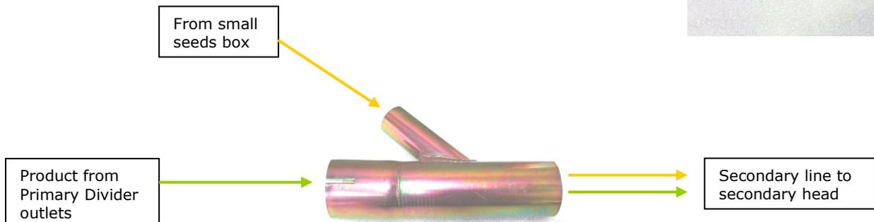
Small seeds induction tubes are a convenient way to place small seed from the small seeds box (option) into the main air streams with the primary product being applied. The blended products then travel via the secondary lines and heads to the sowing boot to be placed in the ground together.
