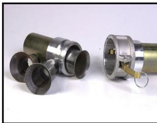
In this case air restrictors should be fitted in the line of the lighter material being sown at the lower rate. The restrictors, fitted in the male side of the camlock breakaways as shown, simply restrict the air flow, stopping the escape of air and keep the system in proper balance.
